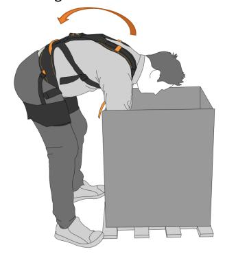
The equipment provides relief of 18 to 28 kilograms, depending on the selected configuration
