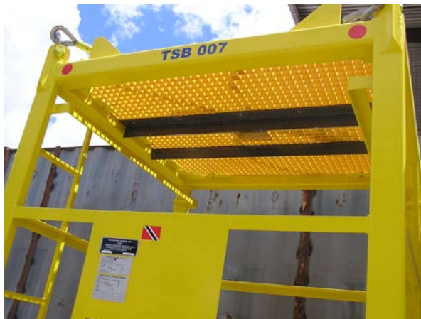
Underside showing stiffeners
