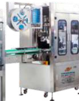
Automatic Shrink Sleeve Label Applicator With Steam Operated Shrink Tunnel
