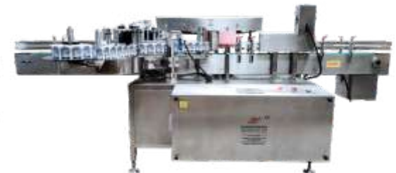
Automatic Sticker Labelling Machine (For Round | Flat Bottle)
