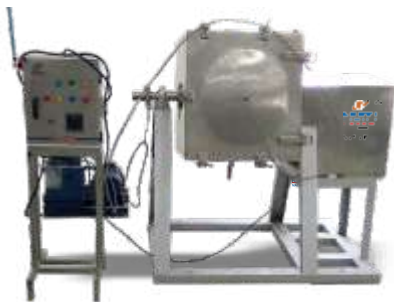
Leak Check In Vacuum Machine
