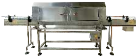
Steam Operated Shrink Tunnel
