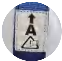
The main hanging point indicator makes the seat belt easier to wear
