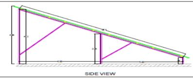
Robot Member Verification: Ok Robot Maximum Reaction in all direction = -13 7KN: Ok Civil Engineer Abdul Kader A.Azhari OEA: 11685
