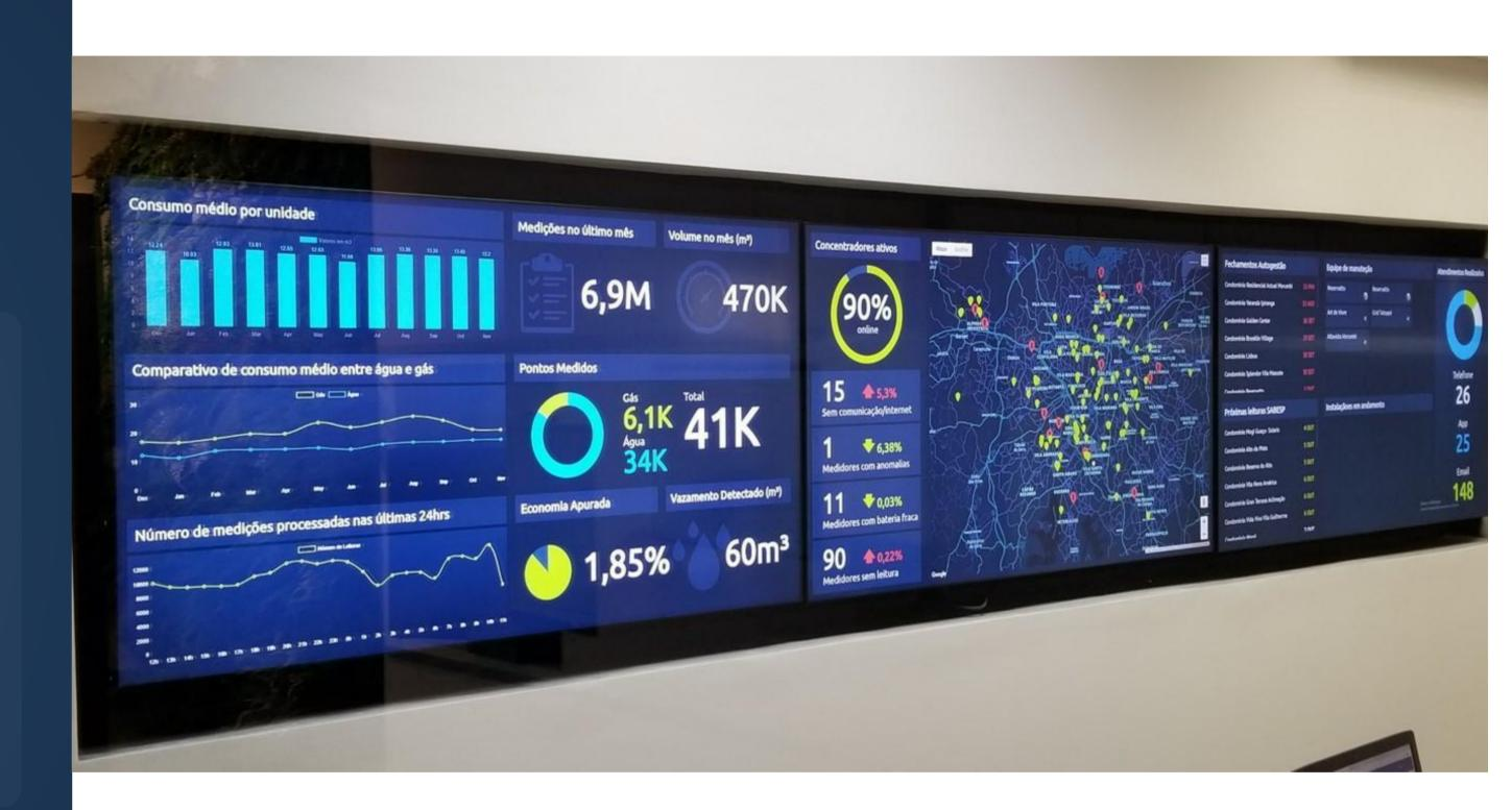
A monitoring and management center tracks measurement information and possible faults and alarms. SMS messages can be configured for emergencies and / or maintenance calls.
