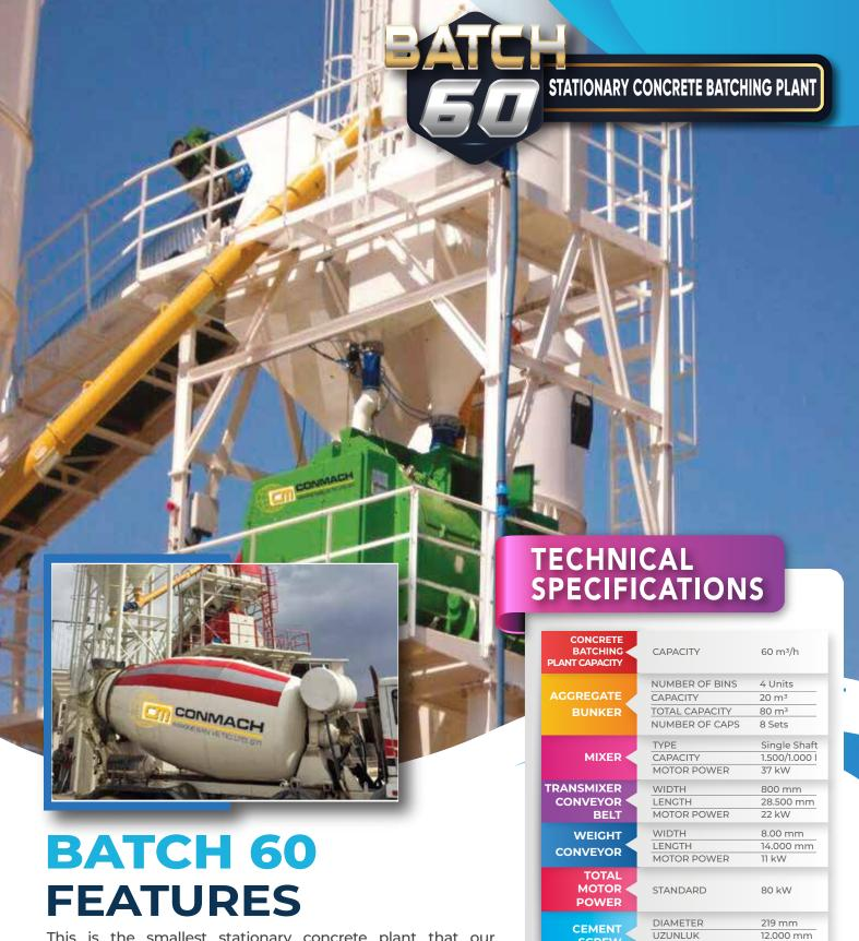
This is the smallest stationary concrete plant that our company produces, and it is capable of producing 60 m³/hour of ready mix concrete. Concrete batching plant is equipped with a single-shaft mixer of 1.500/1.000 L and an aggregate bunker with 4 bins, each of them can take 20 m³ of aggregate materials. It also includes a 1.5 m³ aggregate pre-waiting bunker, 75 ton cement silo with its accessories.
