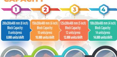
PAVER CAPACITY: 0.55 m<sup>2</sup>/PRESS (550 m<sup>2</sup>/SHIFT)
