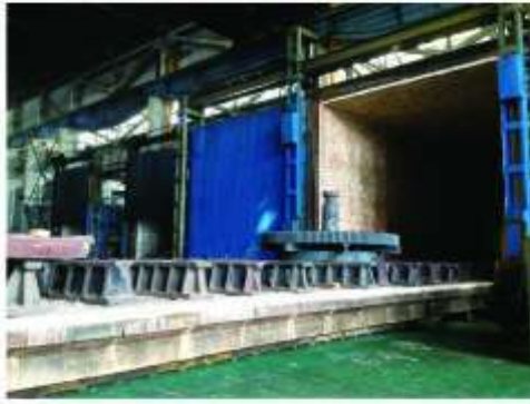
2.6米X5.4米X1.6米台车炉，电加热，最高加热温度1050℃。 Trolley Furnace 2.6m X5.4m X 1.6m electric heating, max temperature is up to 1100℃
