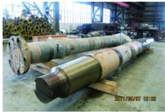
8.9万吨液化气船舵杆 Rudder stock for 89000 ton liquefied gas ship
