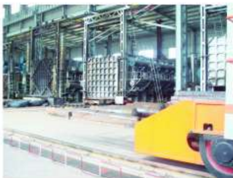
8.6米X4.6米X3.5米台车炉，煤气加热，全电脑控制，最高温度达1100℃。 Trolley Furnace 8.6m X 4.6m X 3.5m gas heating, full computer control, the maximum temperature is up to 1100℃
