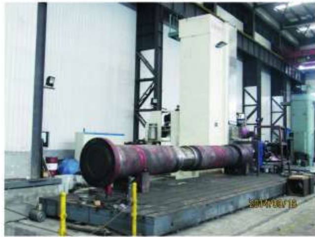
镗床TJK6920A 5m×10m TJK 6920A boring machine 5x10m
