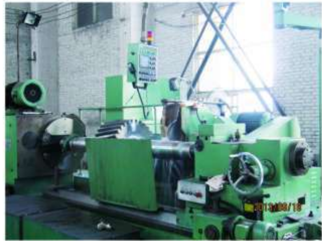
Φ800x5000m程控外圆磨床 Φ800x5000m outer circle milling machine
