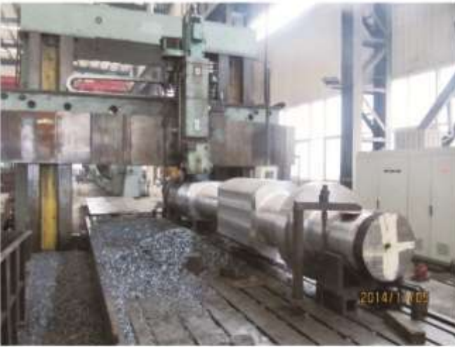
2.2m x 1.8m 数控龙门铣 2.2m x 1.8m CNC gantry milling machine
