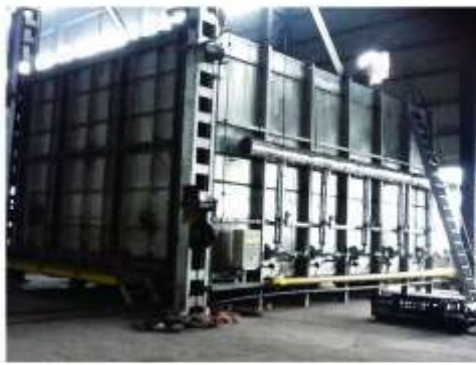
6米 X 13米自动控制台车炉 66m X 13m automatic controlled trolley Furnace
