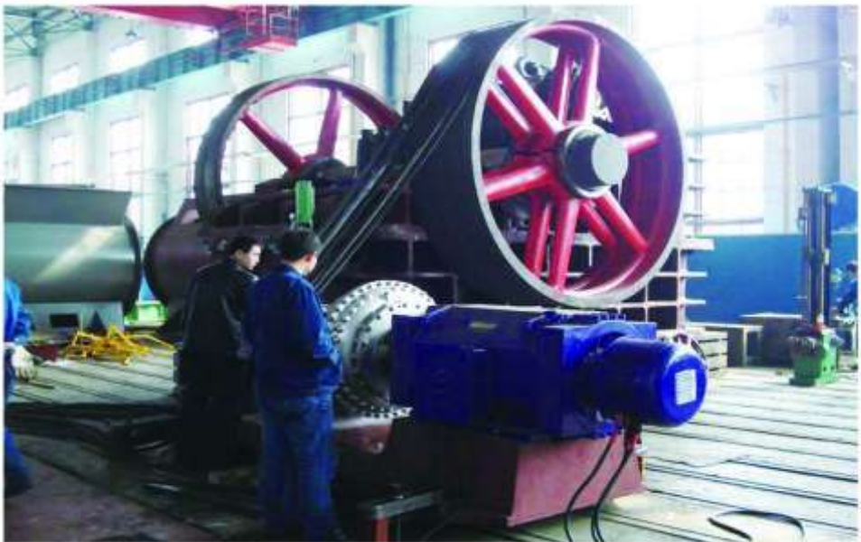
PJ-1200筒摆颚式破碎机 PJ-1200 simple pendulum jaw crusher
