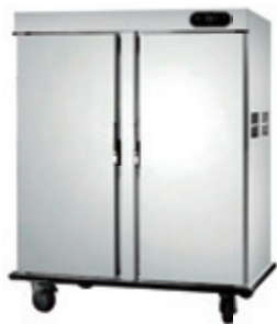
✓ 保温餐车 Food Warmer Cart Model JD-XC102-2 Dimensions(mm):1540x957x1793 Inner size(mm):1350x680x1380 Power supply(KW):2.62 Voltage(V):220 Layer distance(mm):115 Layer Number :22-layer
