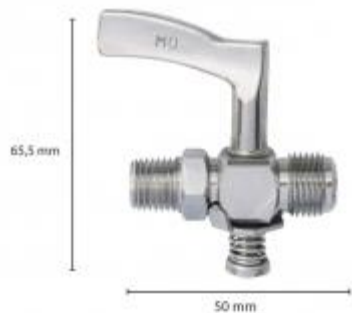
20048 – Chrome Plated Brass Valve 1/4 BSPT x 1/8 BSP x 3/8 SAE
