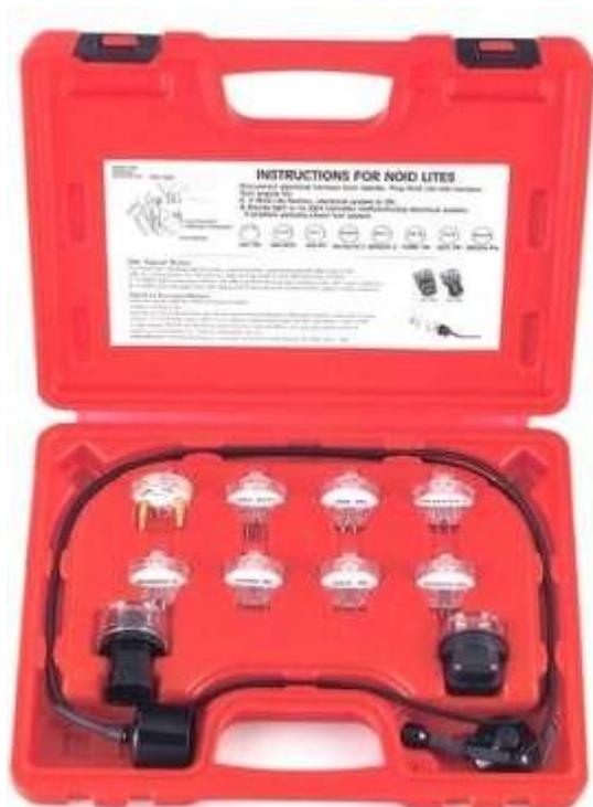
El set incluye 8 "noid lights" para probar GM PFI, FORD TBI, GEO TBI, BOSCH PFI, GM TBI, GM SCPI, GM MULTEC 2, BOSCH 2.
