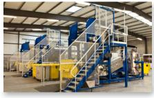
deodorized and filtrated over activated charcoal. The airflow is rejected outside only after this treatment. The treated airflow is of about 250 m3/h. The hopper also includes level indicators (hopper full and hopper empty).
