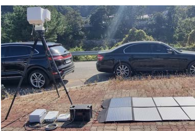
Portable Mobile Base Station
