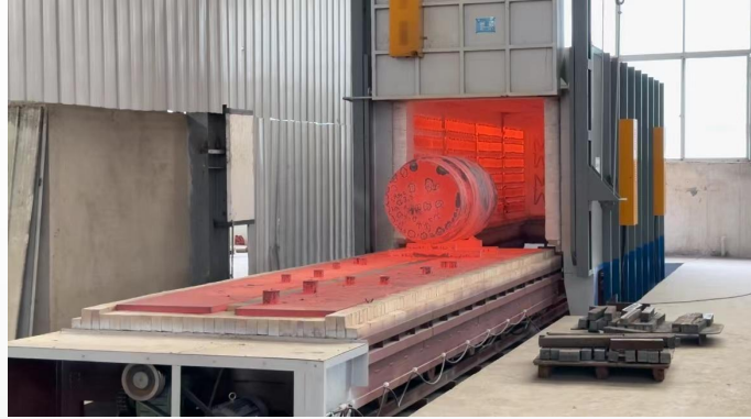
Quenching and tempering heating furnace
