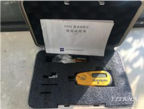
Coating thickness test
