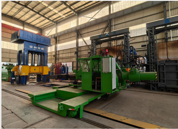
2000 tons fast forging press production line
